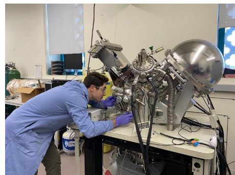
Chris conducts an X-ray photoelectron spectroscopy experiment, which tells us the chemical environments of single atom catalysts. Photo courtesy of Jing Gu.
