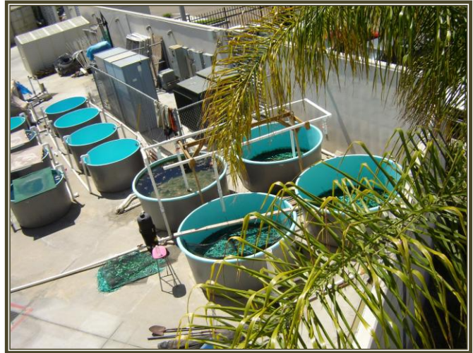
Outdoor research aquaria connected to the flow-through seawater system at the Coastal and Marine Institute Laboratory
